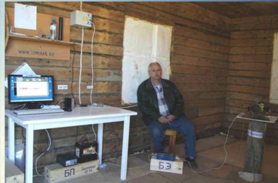
**The position of magnetometer is 6 km away from main village. The quartz sensors is operate without special demands at temperatures from + 50 to - 40 C**
