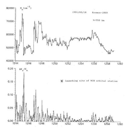
Fig. 2. The electron density onboard observations Kosmos-1809 on 1991/05/18 along the orbit at altitude 950 km above the station MIR take-off: upper panel shows the electron density N: bottom panel shows the relative electron density  $\delta N/N$ .
