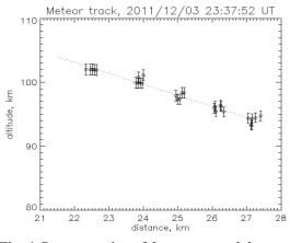
Fig. 4. Reconstruction of the meteor track by triangulation.
