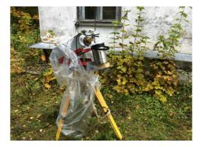
Figure 1. General view of a mobile microwave ozonemeter. Parameters of device: observation frequency - 110.8 GHz; temporal resolution - 15 min; band of the analysis of a spectrometer - 240 MHz; frequency resolution - from 1 up to 10 MHz; in measurements of spectra of a middle atmosphere ozone the method of absolute calibration is used; estimation of a vertical profile of ozone at altitudes from 20 up to 60 km is carried out accuracy o 10 -15%.
