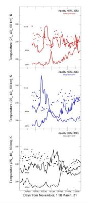
**Figure 2.** Vertical profiles of temperature at separate heights 25, 40 and 60 km (MLS/Aura data).
