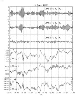
**Figure 1.** The geomagnetic field variations on GOES-14 spacecraft (radial, azimuthal and field-aligned component), goemagnetic field variations in GILL station (X, Y, Z components).
